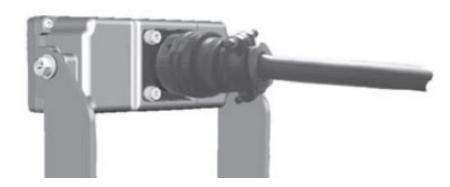
Make any final adjustments to the viewing angle and tighten all bolts. The recommended camera bolt torque specification in between 17 and 20 inch pounds.
